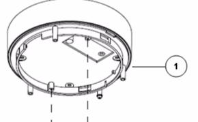
Figure 2-5 Attaching the Camera to the Base Plate
